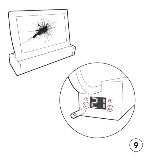
Logicor Clear Heater panels are made from toughened glass but **if the surface of any heater becomes damaged in any way please turn the power off immediately** using the switch located on the bottom right of the panel and contact Logicor for a replacement.
